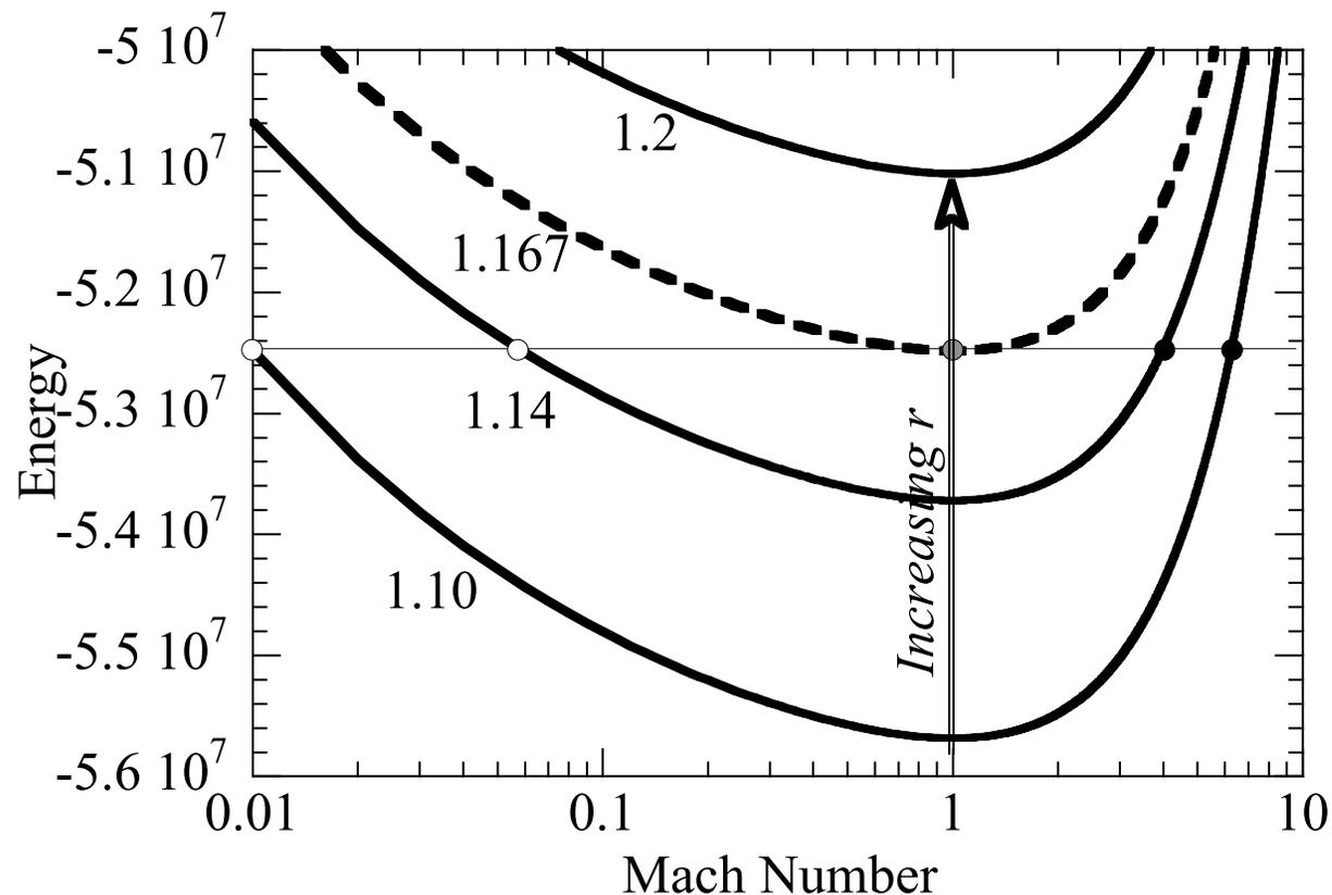
You run out of energy at the sonic point. This is a generalization of the finite depth of a hydrostatic, adiabatic atmosphere
